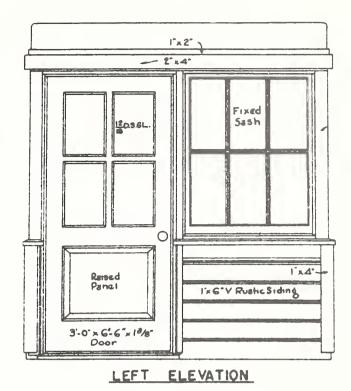
Figure 68. This standard wood lookout house, 7 feet square, was designed in 1934 for use with towers. In this version, without a catwalk, no shutters were provided.
